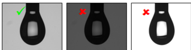
Fig. 7: Drop image with suitable (A), too dark (B) and too bright (C) background illumination.
