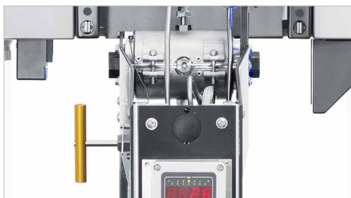
Sample positioning with closed pressure chamber
