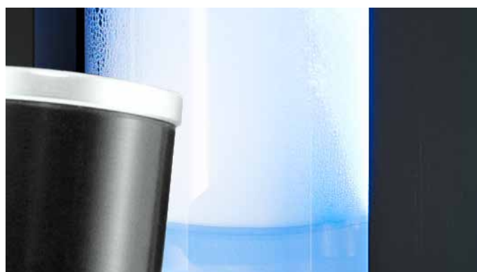
Detection of liquid-foam-boundary
