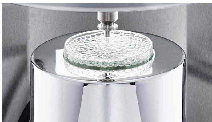
Sample stage with integrated temperature control
