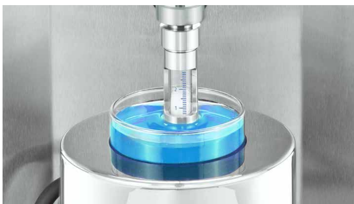
Washburn method for powder contact angle measurement
