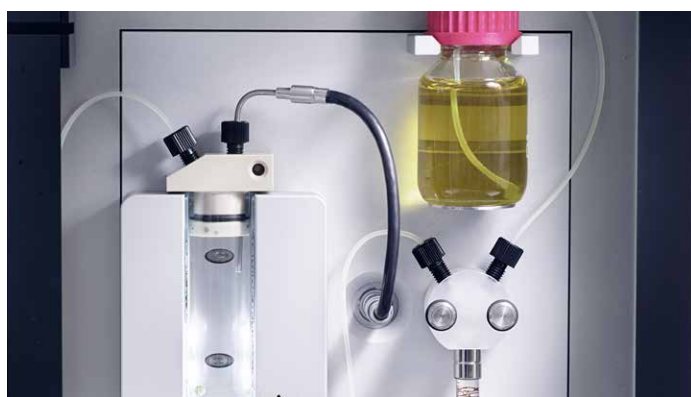
Fully automatic liquid dosing for investigating two-phase systems
