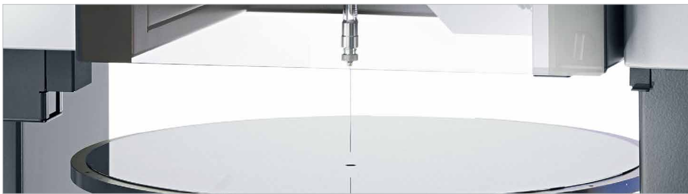
Fully automated drop positioning on a wafer
