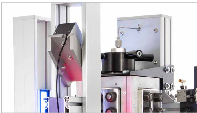
Camera recording foam structure
