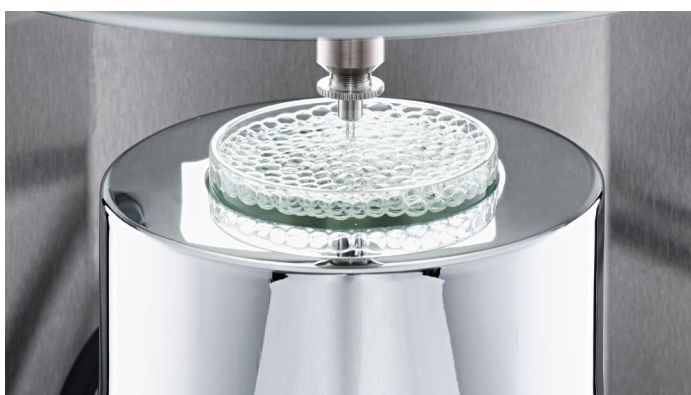
Sample stage with integrated temperature control
