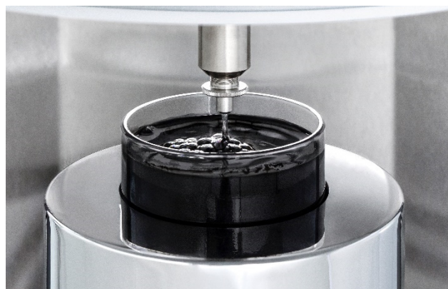
Figure 1: Measurement of dynamic surface tension of an ink with a BP100 Bubble Pressure Tensiometer.
