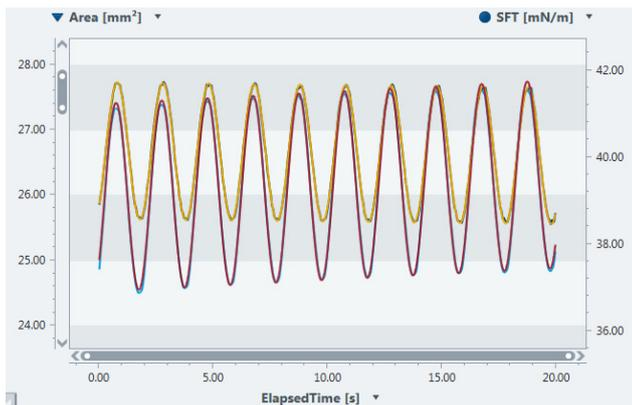
Fig. 2: A drop's area oscillation (dark blue) and resulting SFT (light blue) for sample 1 with a frequency of 0.5 Hz and a frequency amplitude of 3.6%. The adjusted sine functions are also illustrated (area oscillation in yellow, and resulting SFT in red).
