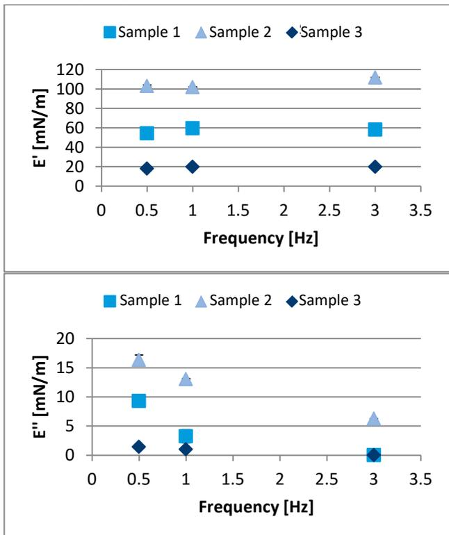
Fig. 3a (above), 3b (below): Elastic modulus  $E'$  and viscous modulus  $E''$  as functions of the vibration frequency for all three samples examined. The amplitude of the surface deformation is  $3.6 \pm 0.4\%$ .
