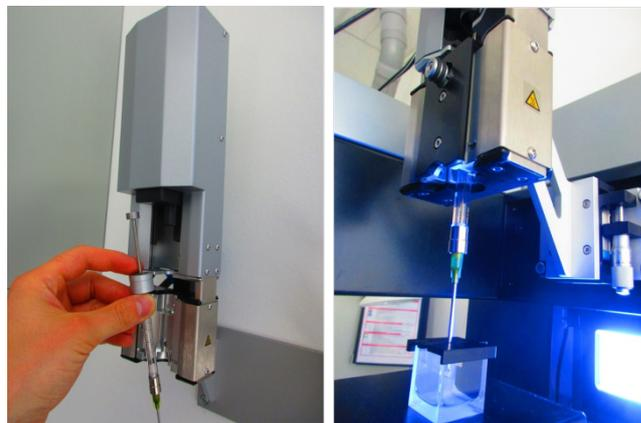
Fig. 1: Experimental setup of the DSA100 with the Oscillating Drop Module – ODM. Left: The filled syringe is inserted. Right: Ready-to-measure setup with the syringe fixed.
