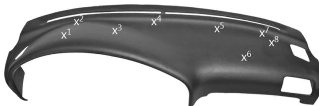
Fig. 3: Schematic representation of a sample dashboard cover. In each case, measurements were carried out at eight spots, which are marked accordingly here.
