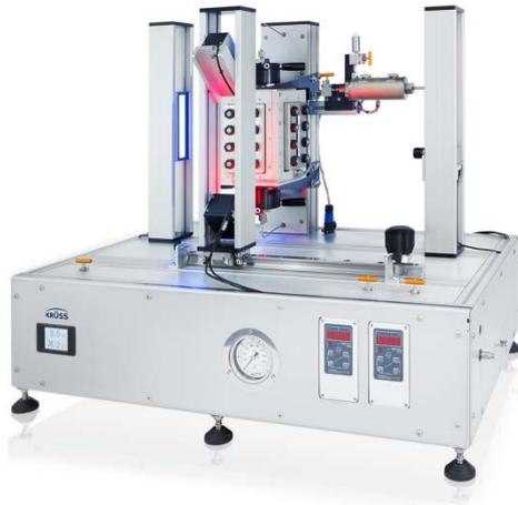
High Pressure Foam Analyzer – HPFA for foam analyses under oil reservoir conditions
