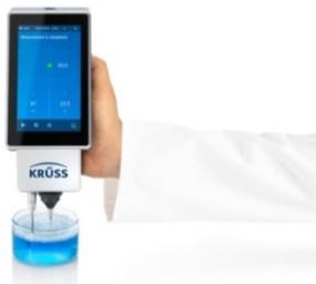
Bubble Pressure Tensiometer – BPT Mobile for quality control of industrial baths containing cleaning or wetting agents
