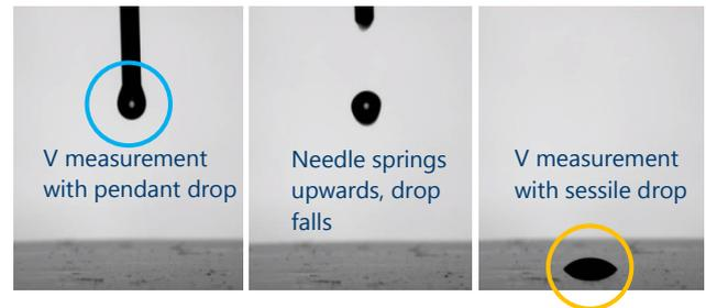
Fig. 2: Test sequence during the volume check
