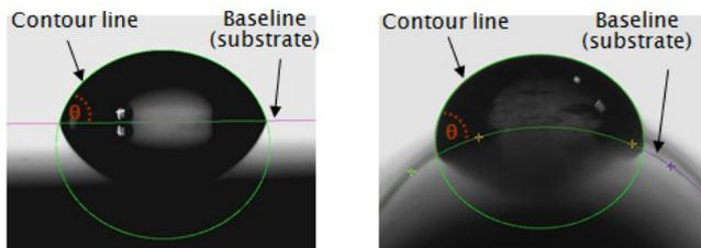
Fig. 4: Contour analysis on a flat and a curved sample surface
