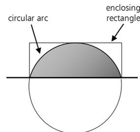
Fig.5 Circular and height-width methods: drop shape as arc
