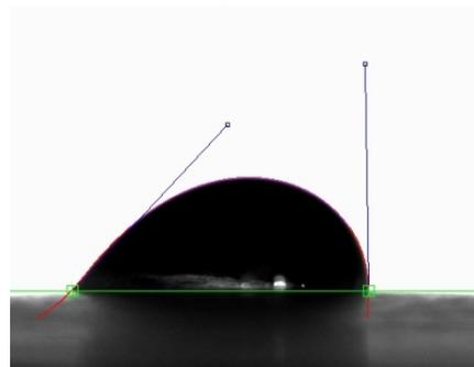
Fig. 7: Polynomial fit with a tilted table measurement. The drop shown is located on an inclined surface.
