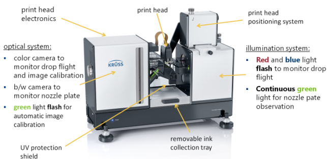
Fig. 1: Construction of the DSA Inkjet with fitted print head
