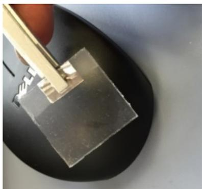
Fig. 2: Adhesive compound with 12% acrylic acid content on cover slip on an SH0601 clamp sample holder for the K100 after measuring in water
