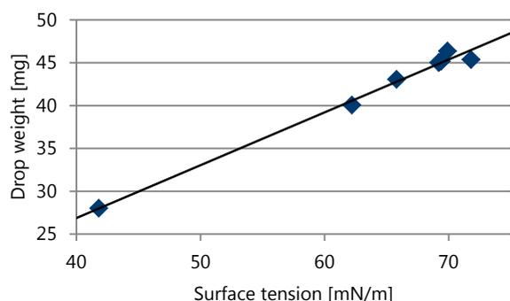
Figure 2: Drop weight of ophthalmic solutions as a function of surface tension as adapted from data published by Van Santvliet and Ludwig [1, 4]. The coefficient of determination  $R^2$  for the linear regression is 0.989.
