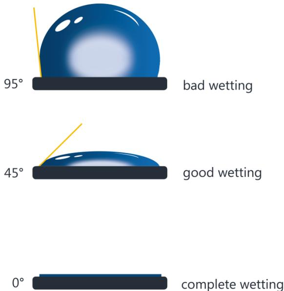
Fig. 2: Relationship between contact angle and wetting
