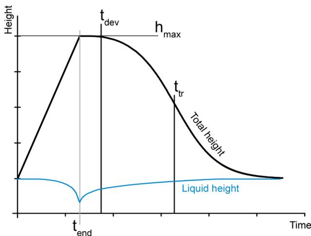
Fig. 4: Determining the foam generation and decay processes using the heights  $h$  and  $h_l$ .
