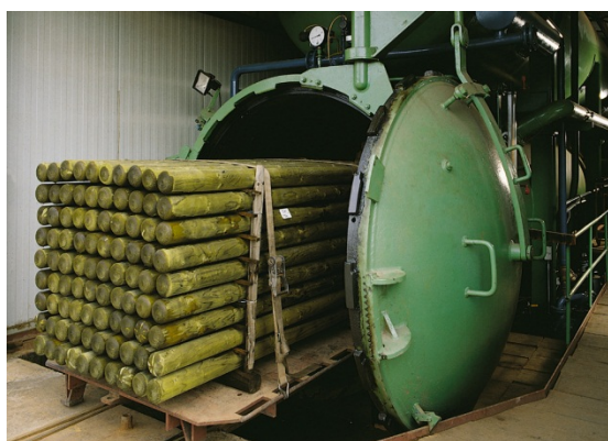
Treated wood leaving a pressure container (photo: Dr. Wolman GmbH)
