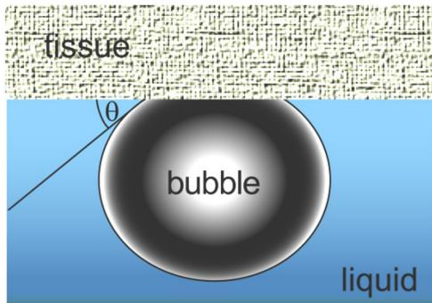
Fig. 1: Schematic view of the captive-bubble arrangement
