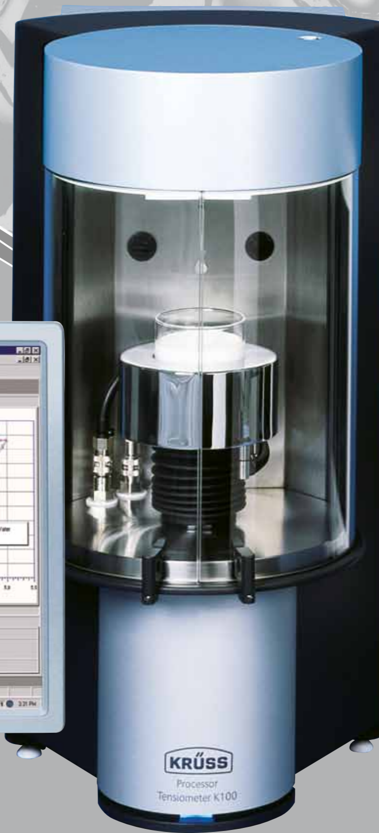
▶ Surface energy determination on single fibre and bundles of fibres
