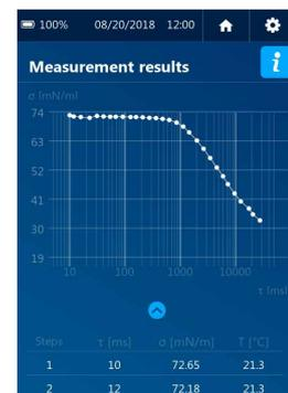
Monitoring and dynamic measurement with BPT Mobile
